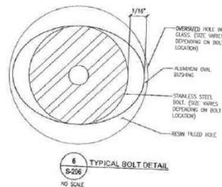
Figure 8: Typical Bolt / Oval Bushing Detail
