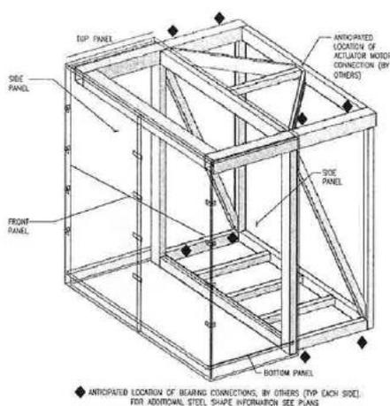
Figure 2: Isometric view of Steel Frame and Glass
